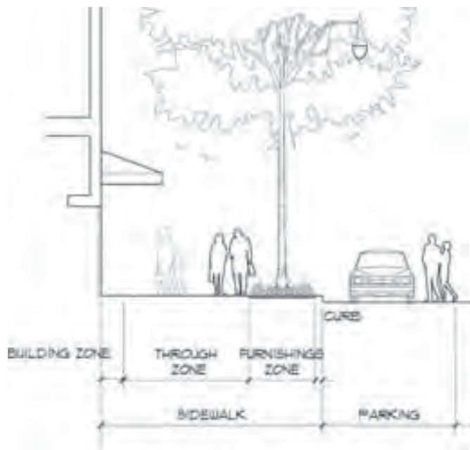
Figure 4 Typical Sidewalk Section
